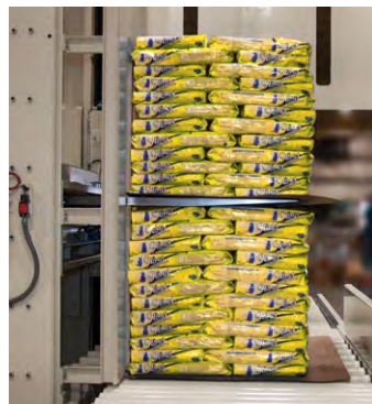
Load stacking system for slip sheets.
