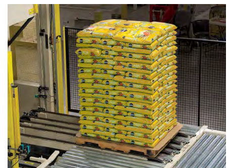
Roller/chain transfer for proper load flow orientation.
