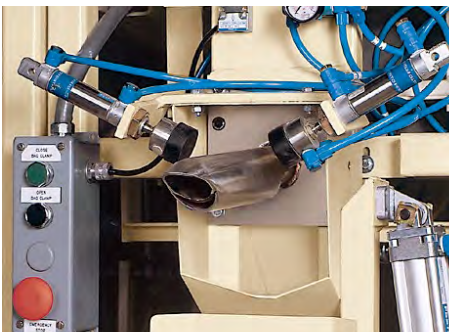
Bags are automatically placed over the nozzle for filling.
