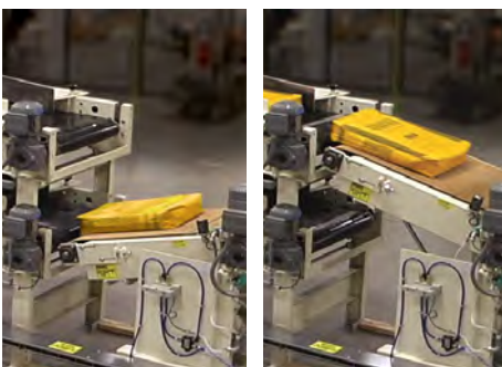
A pivoting conveyor feeds accumulated product from multiple lines into the dual stacking palletizer.
