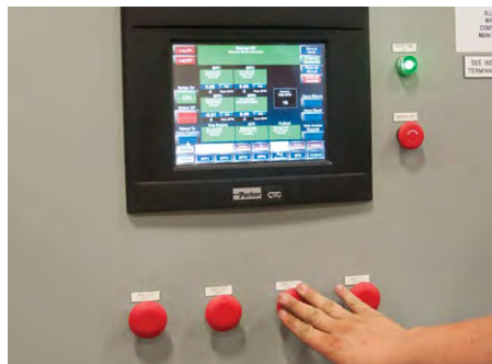
Four in-line packers are controlled independently within the main control panel.
