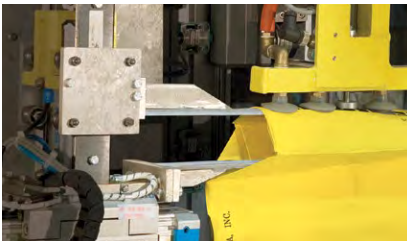
Conveyorized bag feeder provides a steady supply of bags to the packer.
