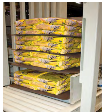
Load stacking system for partial loads.
