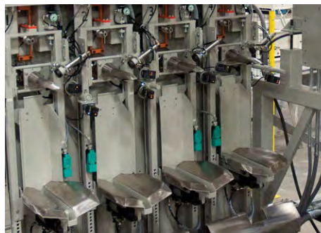
Up to four in-line spouts per bag filling cell.
