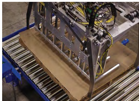
Robotic arm accurately positions pallets onto conveyor for case positioning.
