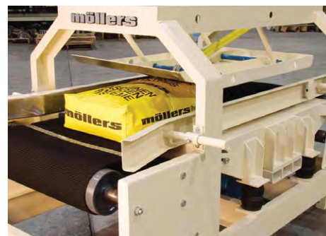
Bag equalizer flattens air-tight, sealed bags.
