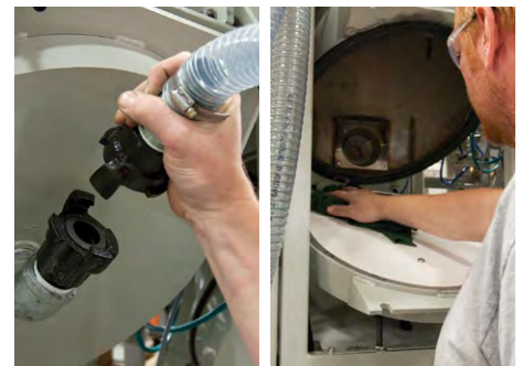
Stainless steel hopper has quick disconnect fittings and drop-down bottom for easy cleaning.
