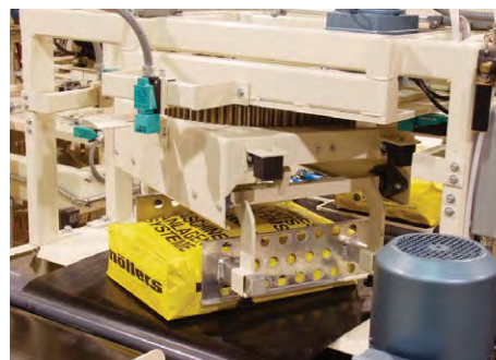
Overhead flap turning device handles up to 30 bags per minute.
