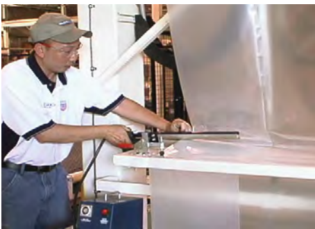
Splicing table with clamps folds down allowing fast and easy film roll splicing.
