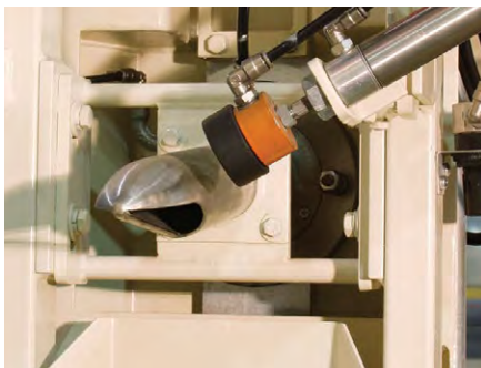
Nozzle with bag detection device.
