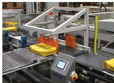
Side reject station automatically removes bags that do not meet proper tolerances.
