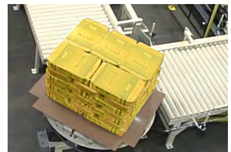
Heavy-duty turntable live roller with all rollers chain driven.
