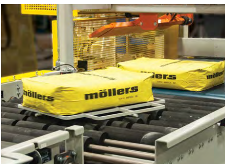
Pop-up turning device handles up to 25 bags per minute.
