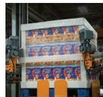
The flaps of the 'Top Cap' are folded with the application of the Stretch-Hood, securing the upper portion of the corner boards
