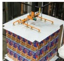
The 'Top Cap' is applied to the load as a top-sheet with 'flaps' prior to entering the Stretch-Hooder
