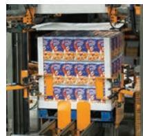
The flaps of the 'Bottom Cap' are folded upward with vertical pneumatic plates to secure the lower portion of the corner boards
